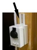
7. Slide motor onto Wall Bracket and lock in place using Latch at top of Motor. **Leave seven (7) ladder slots visible above motor** for future adjustment.
